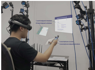
Figure 2: The hardware setup of our interview. A magic leap AR headset and a Huawei P20 were used. They were tracked by OptiTrack.
